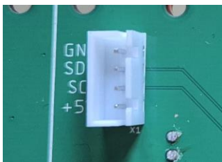
Figure 1 - I2c connector, detail
